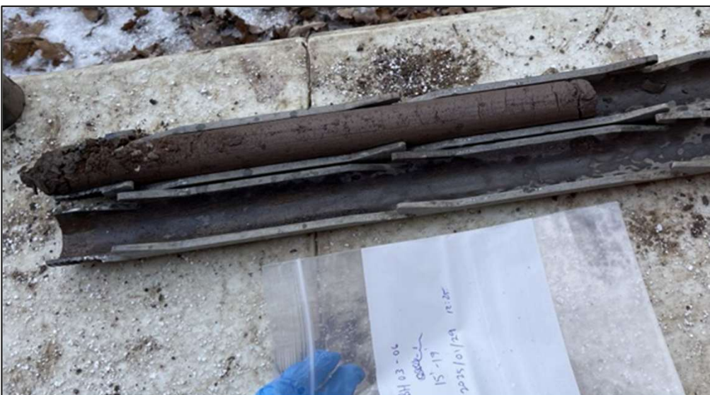
Photo 6: Core sample of BH-03-06, depth 15'-19'.
