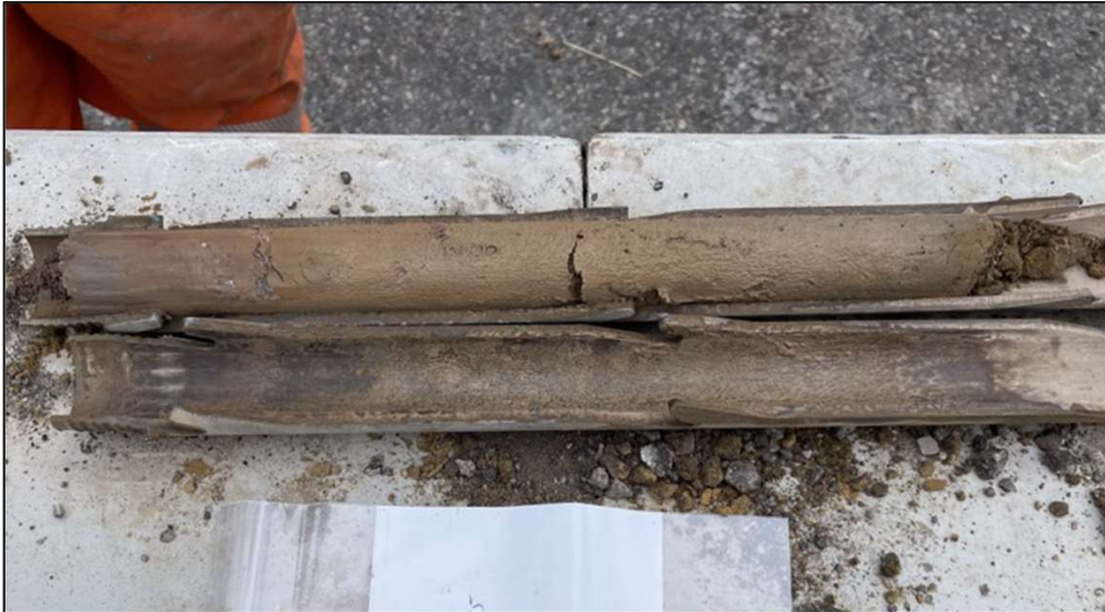
Photo 7: Core sample of BH-04-04, depth 7.5'-9.5'.
