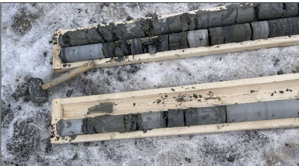
Photo 9: Core sample of BH-05-10, depth 43.9'-44.7'.
