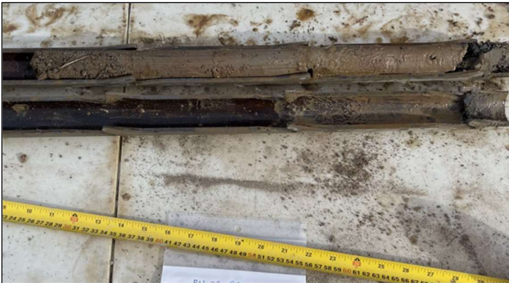
Photo 4: Core sample of BH-02-04, depth 7.5'-9.5'.
